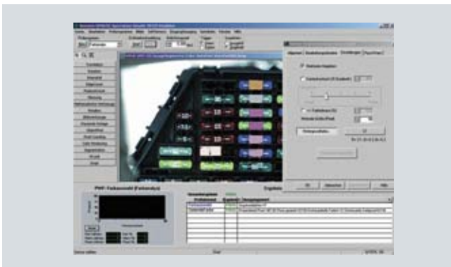
Example for color analysis: Assignment, segmentation and preprocessing of objects of different colors, e.g. for checking the presence/type of automobile fuses
